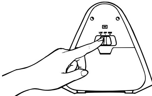
To turn swing off, slide switch to the center OFF position.
